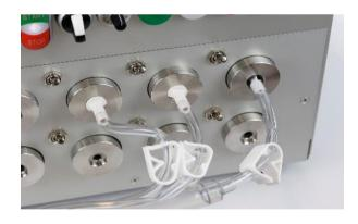
Each tube connector is placed in its own type of coupling, clamped and closed off, so that there is no leakage between the connector of the design and the coupling of the test cabinet.
