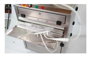
The Flexible Bag Integrity Test Unit 2D (FBITU-2D) is designed for testing 2D single use flexible bags between restraining plates, used in the Life Science industry.
